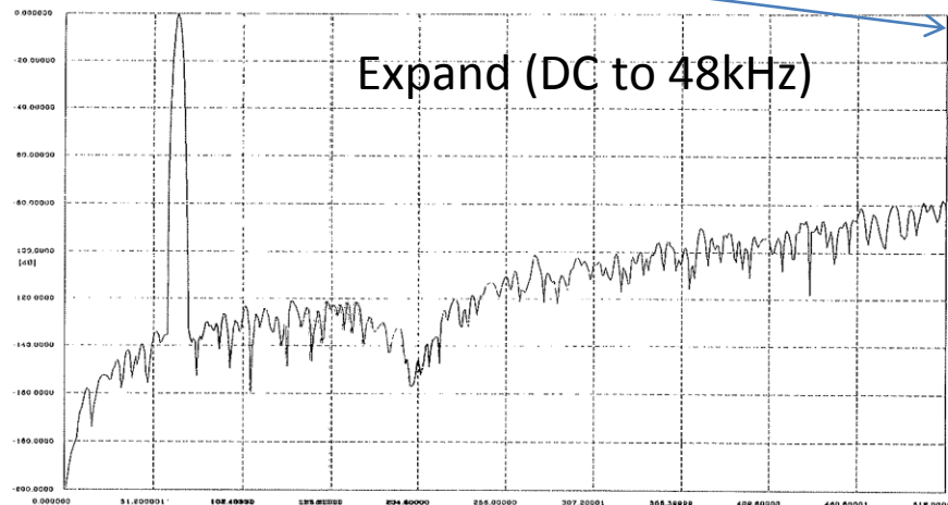
Fig. 7. Expanded simulated modulator output spectrum.
