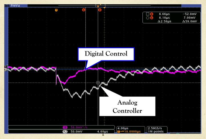
Reduced voltage deviation and faster settling time! Much smaller output capacitance can be used.
