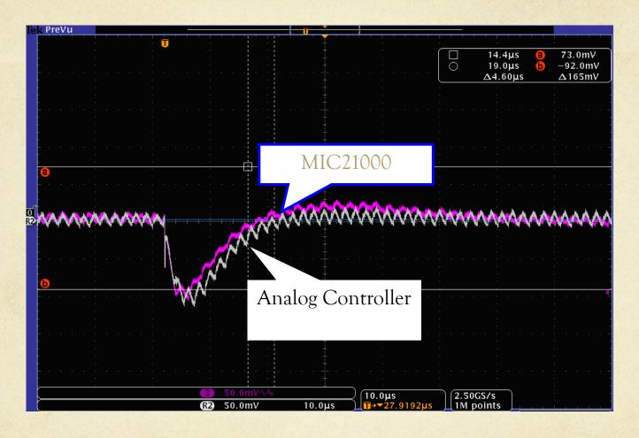
Ultra-Fast Load Transient Response can be enabled by modifying the Digital Filter Coefficients.
